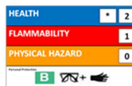
HMIS (Hazardous Material Information System)
